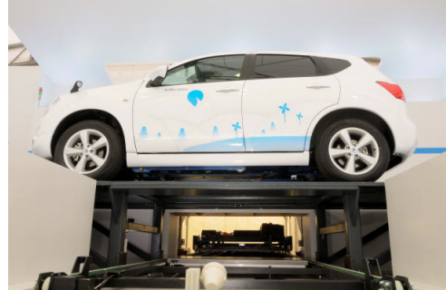
Fig. 1: Battery switching mechanism of "Better Place" company
